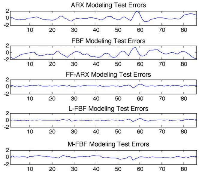
Fig. 3. Box-Jenkins furnace identification testing errors.
